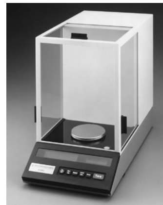
FIGURE 2-3 Electronic analytical balance measures mass down to 0.1 mg. [Courtesy Fisher Scientific, Pittsburgh, PA.]
