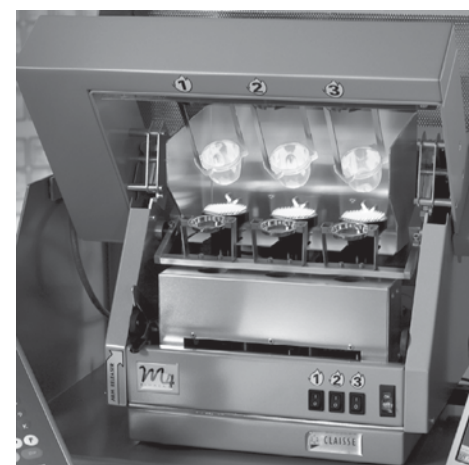
FIGURE 27-8 Automated apparatus that fuses three samples at once over propane burners. The Pt/Au crucibles rotate while they are inclined. [Courtesy Claisse, Quebec.]
