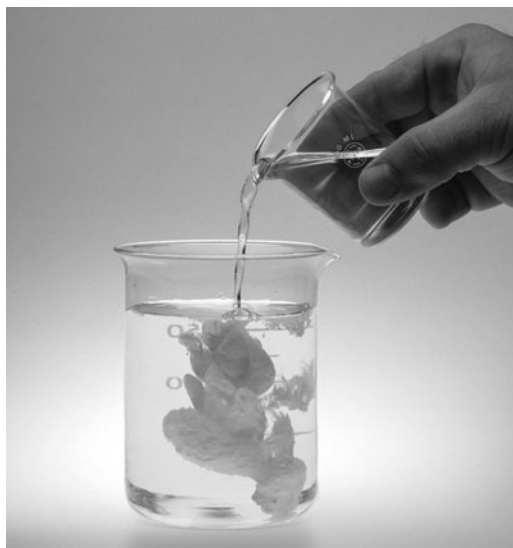
FIGURE 6-2 A yellow solid, lead(II) iodide (PbI 2 ), precipitates when a colorless solution of lead nitrate (Pb(NO 3 ) 2 ) is added to a colorless solution of potassium iodide (KI). [Photo by Chip Clark.]
