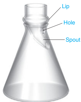
FIGURE 27-11 Reflux cap for wet ashing in an Erlenmeyer flask. The hole allows vapor to escape. The curved spout touches the inside of the flask. [From D. D. Siemer and H. G. Brinkley, "Erlenmeyer Flask-Reflux Cap for Acid Sample Decomposition," Anal. Chem. 1981, 53, 750.]
