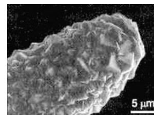
FIGURE 16-16 Boron-doped diamond coating on Pt electrode. [From J. Cvačka et al., Anal. Chem. 2003, 75, 2678. Courtesy G. M. Swain, Michigan State University.]
