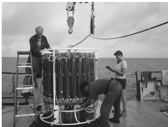
A carousel of 12-L plastic bottles lowered on a Kevlar line from a research vessel is used to collect ocean water without introducing trace metal contamination during collection. Samples are removed from the bottles in a plastic-lined clean room inside a cargo container on the deck of the ship.
