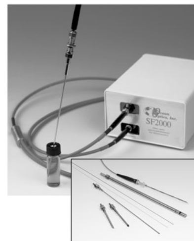
FIGURE 18-22 Fiber-optic sensor measures O_2 by its ability to quench the luminescence of Ru(II) at the tip of the fiber. A blue-light-emitting diode provides excitation energy. Inset shows several probes. [Courtesy Ocean Optics, Dunedin, FL.]
