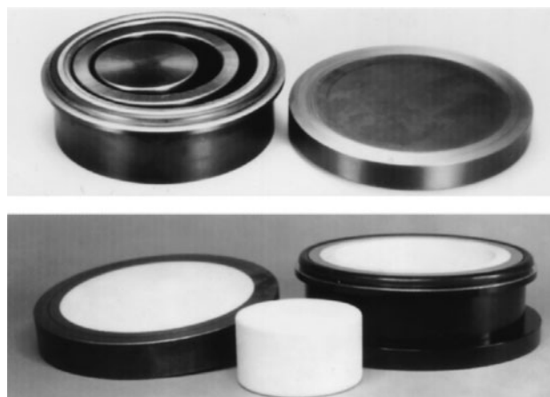
FIGURE 27-6 Shatterbox laboratory mill spins a puck and ring inside a container at high speed to grind up to 100 mL of sample to a fine powder. [Courtesy Spex Industries, Edison, NJ.]
