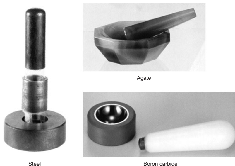
FIGURE 27-5 Steel, agate, and boron carbide mortars and pestles. The mortar is the bowl and the pestle is the grinding tool. The boron carbide mortar is a hemispheric shell enclosed in a plastic or aluminum body. The pestle has a boron carbide button at the tip of a plastic handle. [Courtesy Thomas Scientific, Swedesboro, NJ; and Spex Industries, Edison, NJ.]
