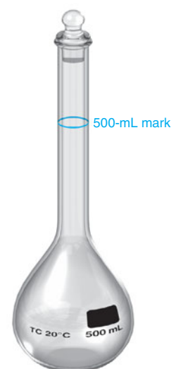
FIGURE 1-3 A volumetric flask contains a specified volume when the liquid level is adjusted to the middle of the mark in the thin neck of the flask. Use of this flask is described in Section 2-5.
